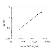
\* The typical standard curve is shown above. This curve can not be used to derive test results. Please run a standard curve for each assay.
