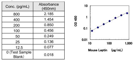
\* The typical standard curve is shown above. This curve can not be used to derive test results. Please run a standard curve for each assay.
