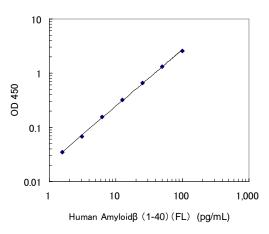
The typical standard curve is shown above. This curve can not be used to derive test results. Please run a standard curve for each assay.
